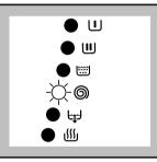
To select **Drain** press the SKIP button three times, the **wash - rinse - spin** LED,s go out.
